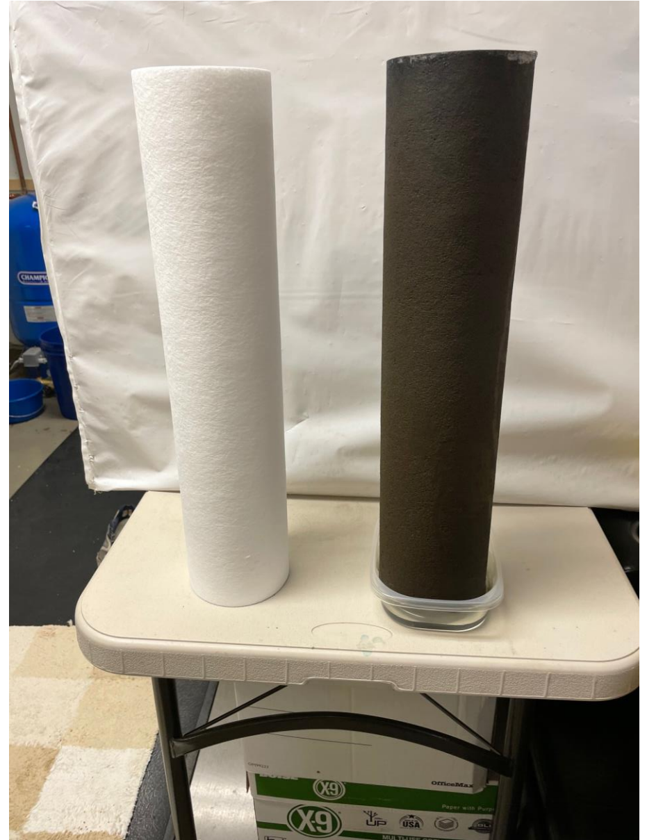
Water quality conditions - Frequent filter changes
